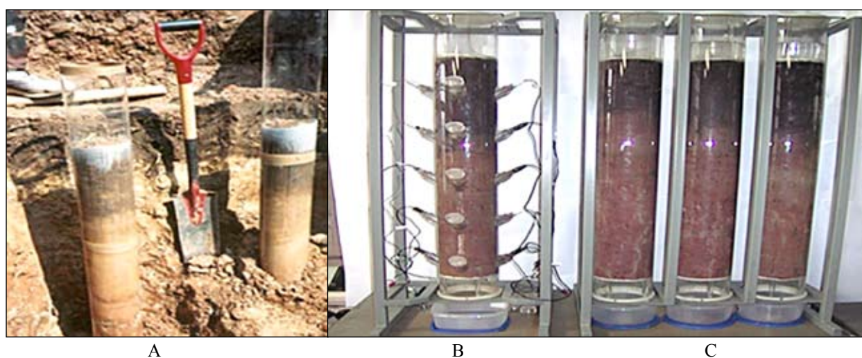
Figure 2. Filling (A) and final stand (B, C) of the model columns of the soil monoliths
